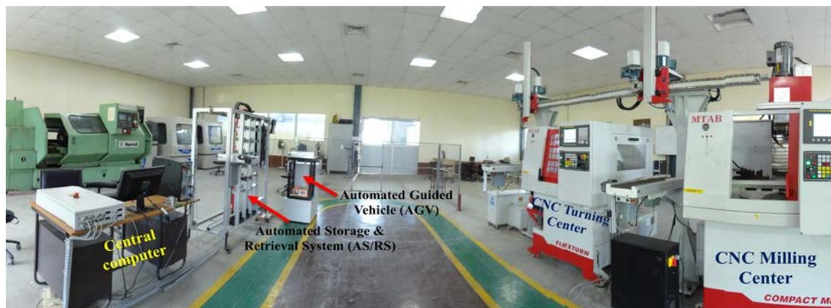
Figure 1.2.4 A FMS Setup
