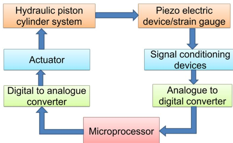
Figure 1.1.6 Microprocessor based equivalent spring mass system
