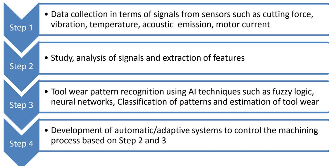
Figure 1.2.3 Steps followed in an indirect tool monitoring system
